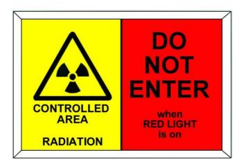
The disadvantage with the 2-stage light is that there may be only a very brief interval between the red portion being illuminated and ionizing radiation being emitted. If the X-ray generator can easily be switched off between cases then the single stage light (duplicated or otherwise) may be more appropriate.
